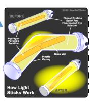
→ thin wall separates two chemicals → when wall is broken the chemicals **mix** and react to **produce** light
